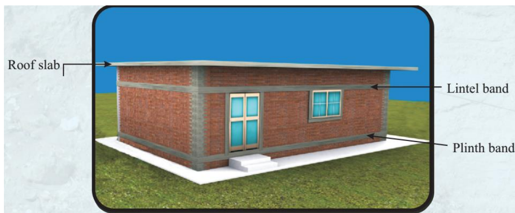
Figure 17-13: Concrete Bands Provided at Specified Levels
